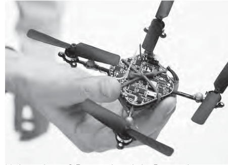
University of Pennsylvania's General Robotics, Automation, Sensing and Perception (GRASP) Lab has developed 'swarms' of autonomous flying nano robots
